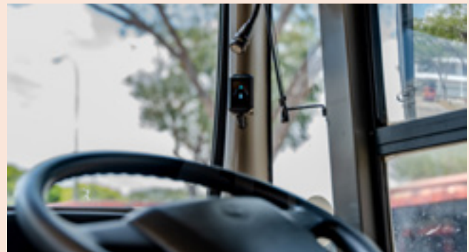
The headway monitoring screen displays the time in seconds to the vehicle in front, and alerts the Bus Captain if the bus moves beyond its current driving lane without signalling its intentions.
