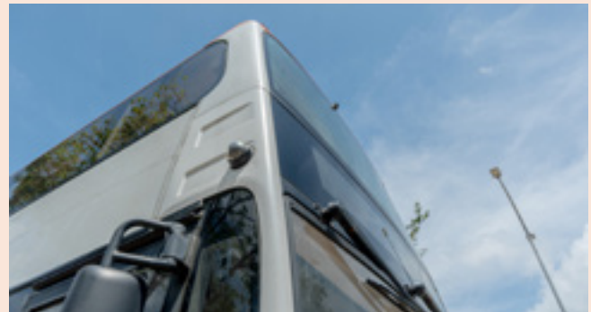
One of four wide-angle field-of-view cameras installed to provide comprehensive coverage of blind spots.
